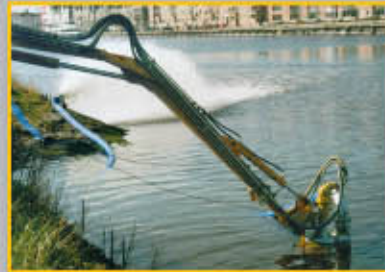
Hydraulic water pump 6500 ltrs/min. (WHP1.SS)
