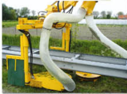
Guard rail mower appropriate for suction (VRMA.SS)
