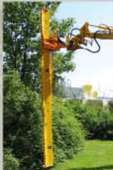
Heavy hedge cutter with double rotation head (HGR300.SS.HW180HK)
