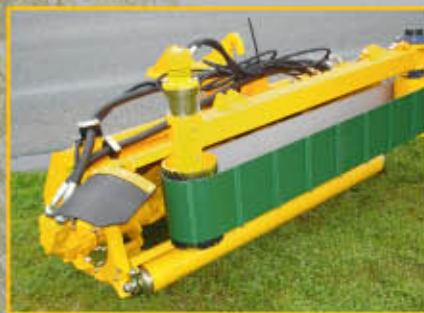
Eco mower with auger unit for suction
