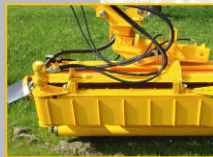
Eco mower with auger unit for suction
