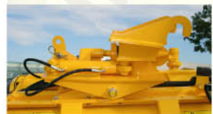
Hydraulic rotation head 90° with mechanical free travel construction (SS.HDP90)
