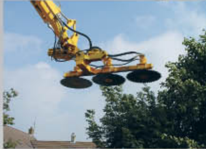
Threefold saw unit with double rotation head (CZH3x75.SS.HD105HK)
