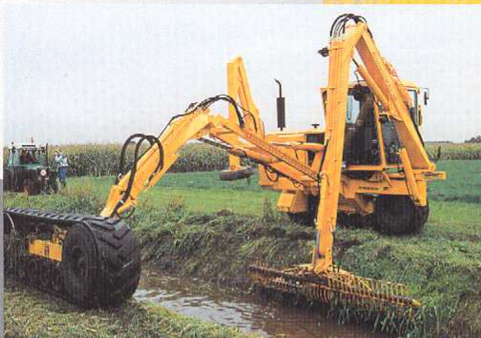
The Pontonnier with mowing bucket, 3 metres
