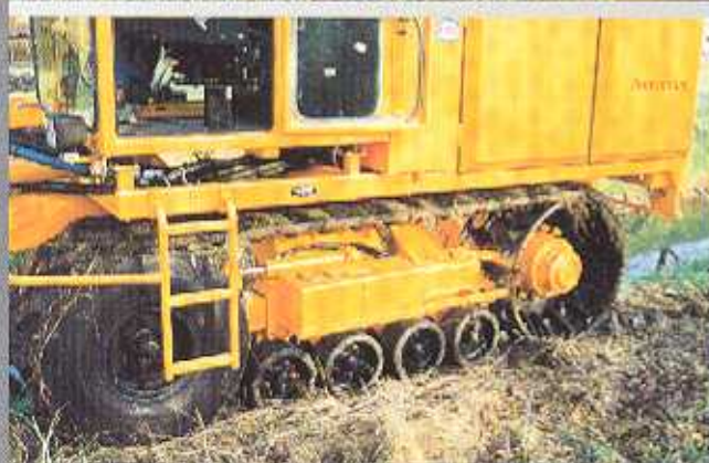
Automatically adjustable heavy wheel mechanism
