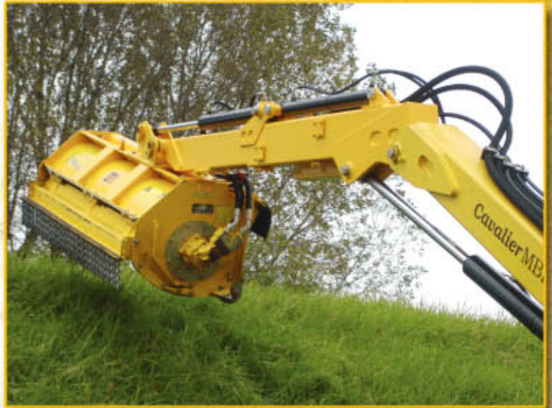
Hydraulic operating sliding boom – slid in
