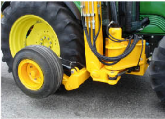
Supporting wheel for more stabilization
